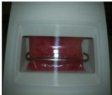
Figure 1. Pulsifier® showing the beating ring
