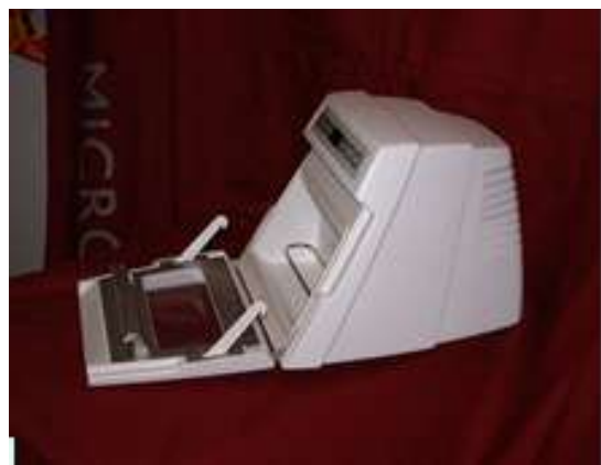
Figure 2. Pulsifier® showing door release for easy cleaning.
